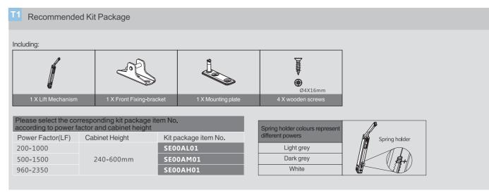
! Front fixing bracket SE00H should be ordered when the front is narrow Alu frame door.
