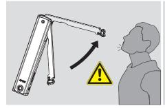
The arm of this device could spring up and cause injury!
