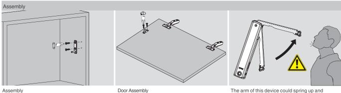
The arm of this device could spring up and cause injury.
