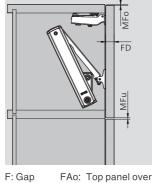
FAo: Top panel overlay MFu: Bottom Min. gap MFo: Top Min. gap
